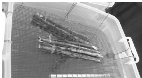
Figure 2: Kenaf water retting process.
