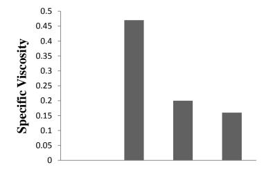
Fig 4: Effects of Mercerization Processes on the Specific Viscosity of Fibres Retted with NaOH and Na<sub>2</sub>SO<sub>3</sub> for 10 mins.
