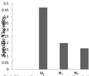
Fig 2: Effects of Retting Processes on the Specific Viscosity of Fibres Retted with NaOH and Na<sub>2</sub>SO<sub>3</sub> for 10 min.
